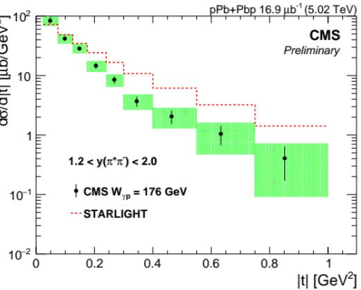
bins together with the STARLIGHT prediction] Differential cross section  $d\sigma/d|t|$  (full circles) in four different rapidity bins. The error bars show the statistical uncertainty, while the shaded areas represent the statistical and systematic uncertainties added in quadrature. The dashed lines show the STARLIGHT predictions.
